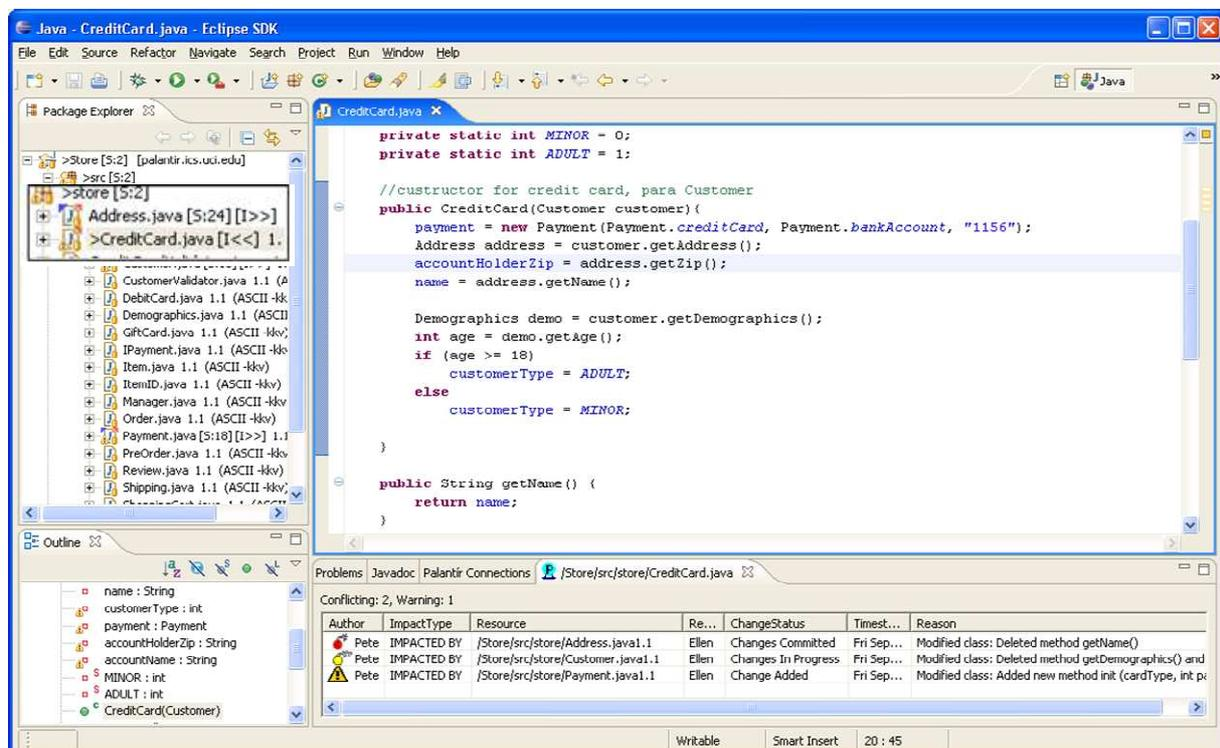
**Figure 2 Palantír screen shot: blue and red decorators indicate concurrent changes in documents in different severity levels.**
