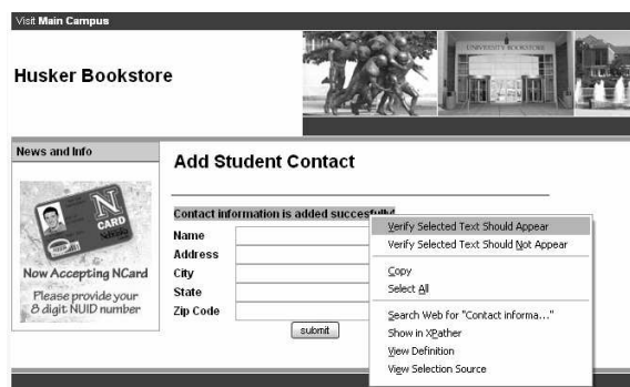
Figure 2: Manual assertions are entered via context menus that allow users to verify whether selected text should appear or not.
