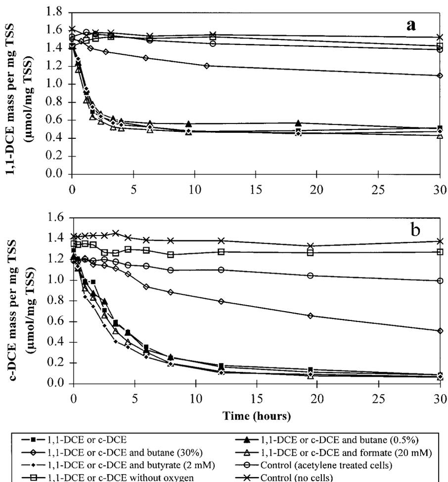
FIG. 1. Resting Cell Transformation of: (a) 1,1-DCE (3.4-mg TSS used); (b) c-DCE (4.5-mg TSS used) in Presence or Absence of O<sub>2</sub>, Butane, Butyrate, or Formate
