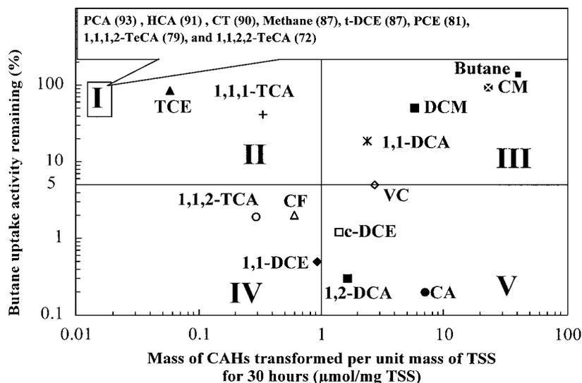
**FIG. 3. Mass of CAHs Transformed per Milligram TSS after 30 h of Incubation versus Butane Uptake Activity after Exposure [Values in Class I Box (No Transformation) Indicate Percentage of Butane Uptake Activity Remaining after Exposure to Each Compound]**
