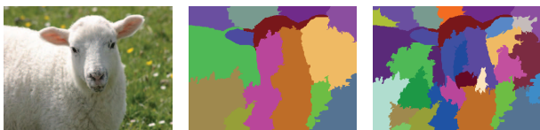
Figure 2. Example image to illustrate regions of homogeneous appearance. Left: original image. Center: segmentation by the original algorithm [9]. Right: segmentation by our modified algorithm. Over-segmentation of an image is desirable for Spatial-LTM because regions can easily be merged into the same topic during learning.
