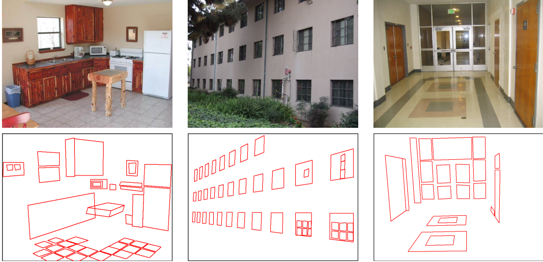
Figure 38: Some experimental results. The first row shows the input images. The second row shows the computed rectangle configurations. From [31].
