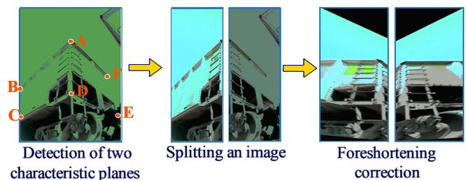
Figure 2. Perspective correction by specifying two planes A-B-C-F and A-E-D-F. As the final result, two views of the car are obtained, as if two cameras perpendicular to the side and end of the car were available
