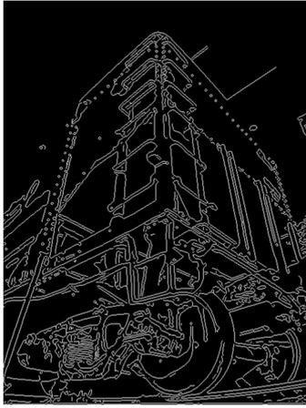
Figure 8. Images showing the edges detected on the corner of a freight car illuminated at night.
