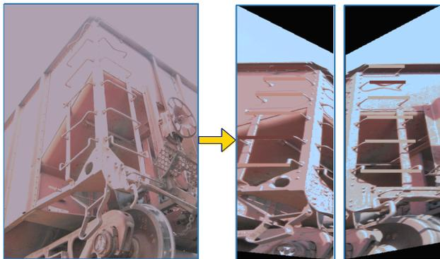
Figure 3. Detection of ladder rungs and handholds; yellow indicates no exception and red indicates deformed appliances
