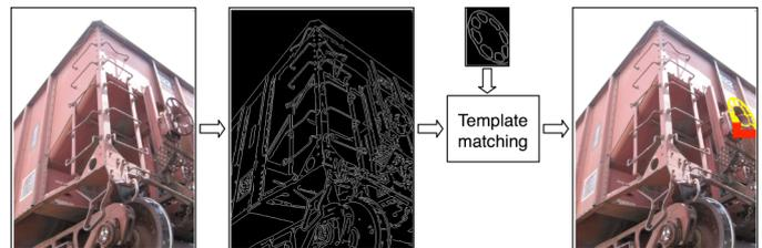
Figure 4. Brake-wheel detection; yellow indicates no exception and red indicates deformation of the brake-wheel
