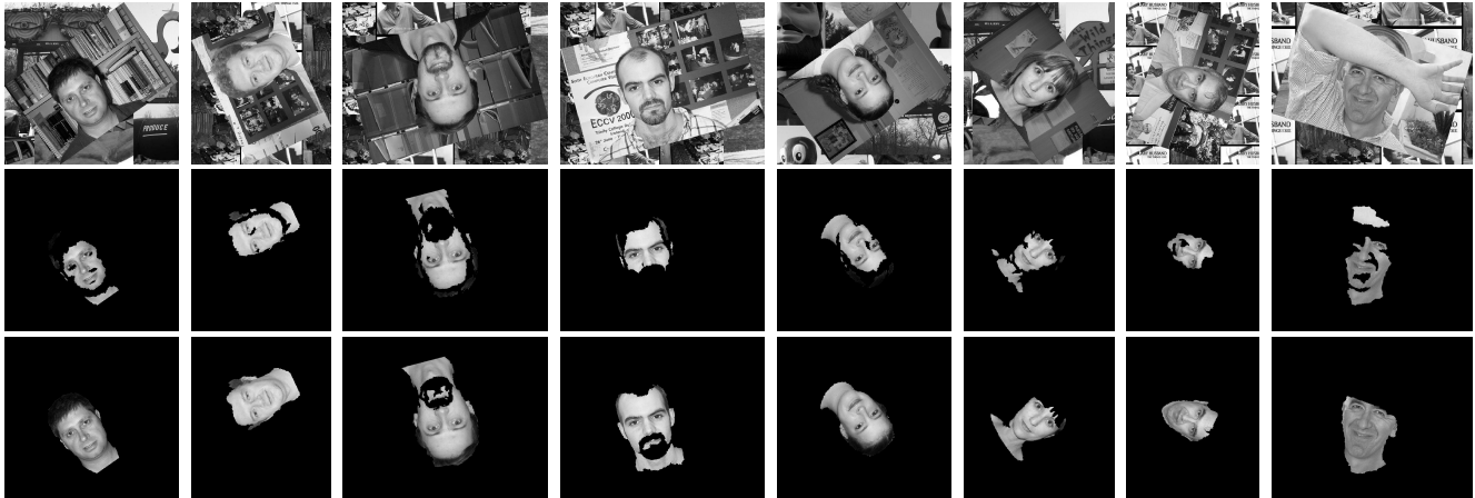
Figure 3. Detection and localization of Caltech faces : (top row) randomly rotated images; the results are obtained when the model is learned on M/2=3 (middle row), and M/2=6 (bottom row) positive training images, and for the highest F -measure. The training set did not contain a bearded face.
