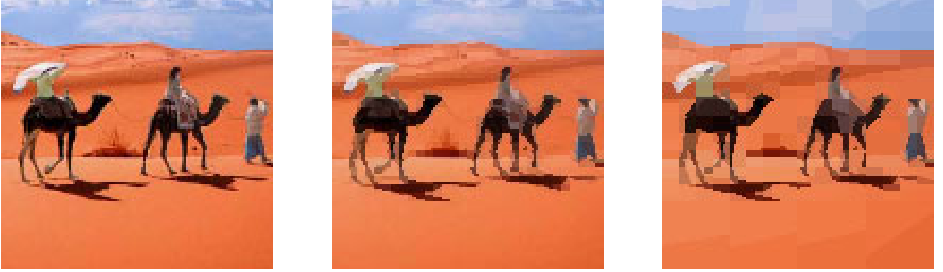
Fig. 3. The MLDA representation: (left) original image, (center) no pruning 1024 leaf nodes, (right) with pruning 253 leaf nodes
