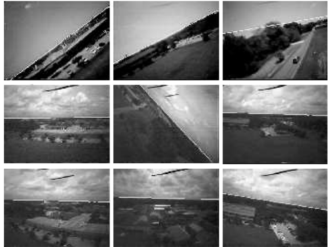
Fig. 8. Various horizon-detection examples under different lighting conditions (sunny and cloudy) and with varying degrees of video-transmission noise. For each example, the white line indicates the algorithm's horizon estimate.
