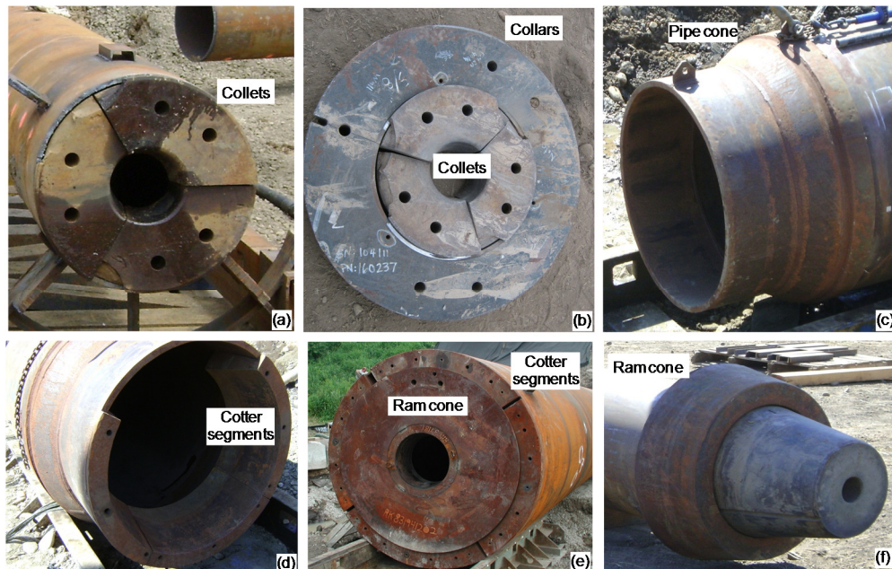
Figure 2. Typical set up of pipe ramming installation project.
