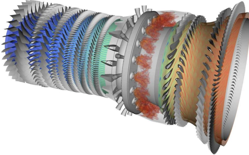
FIGURE 6. Simulation of the full high-spool. Compressor: entropy; Combustor: temperature; Turbine: entropy.
