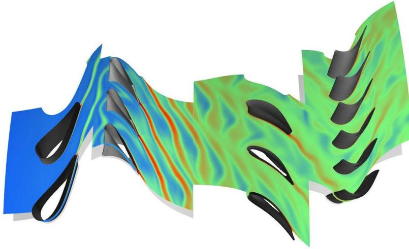
FIGURE 3. Turbine, 20 degrees sector; Instantaneous entropy distribution for the unsteady solution in a radial grid plane for the scaled geometry.
