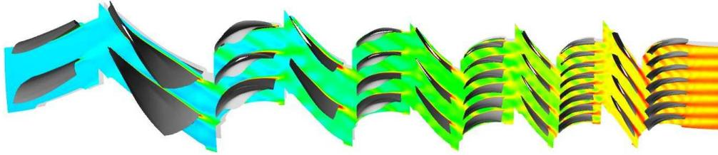
FIGURE 4. Compressor, 20 degrees sector; instantaneous entropy distribution for the unsteady solution in a radial grid plane for the scaled geometry.
