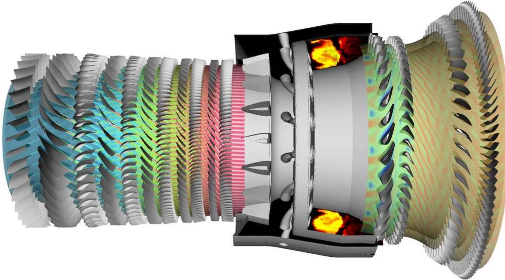
FIGURE 5. Simulation of the full high-spool. Compressor: axial momentum; Combustor: temperature; Turbine: axial momentum.
