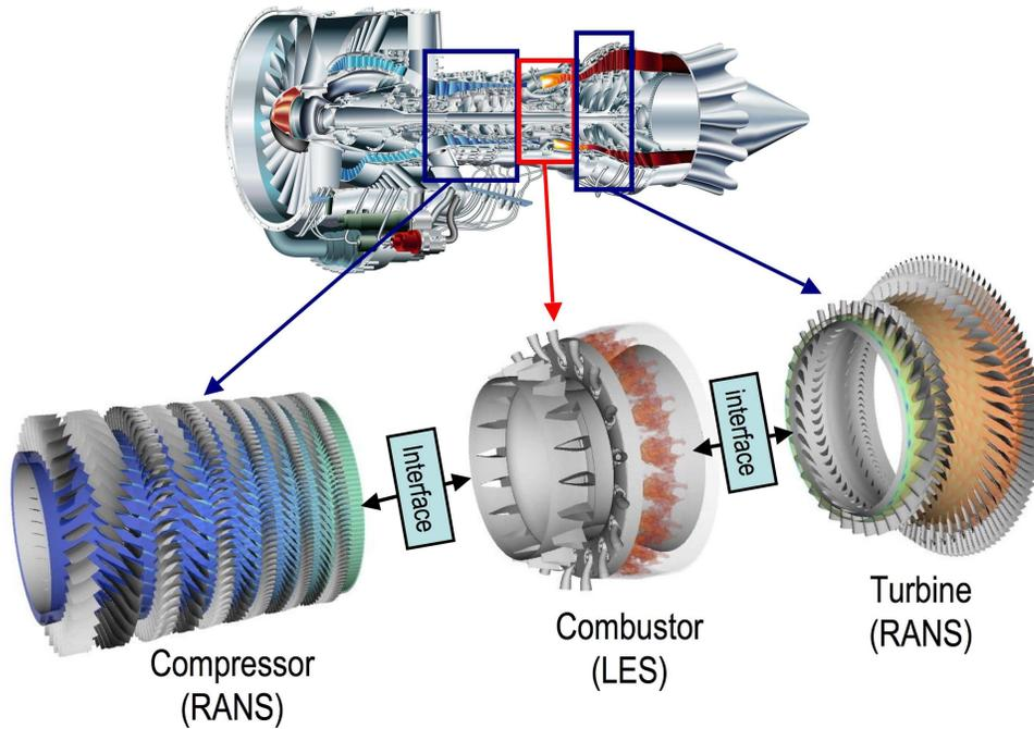
FIGURE 1. Decomposition of the engine for flow simulations. Compressor and turbine with RANS; Combustor with LES.
