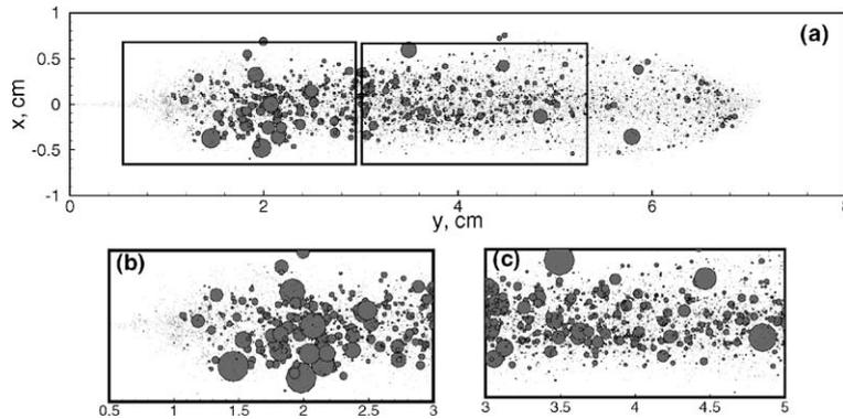
Fig. 8. Instantaneous snapshot of spray evolution using hybrid approach for  $P = 1.1$  MPa. Size of the circles scales with the number of droplets represented by the computational particle: (a) full view, (b,c) close-up views.
