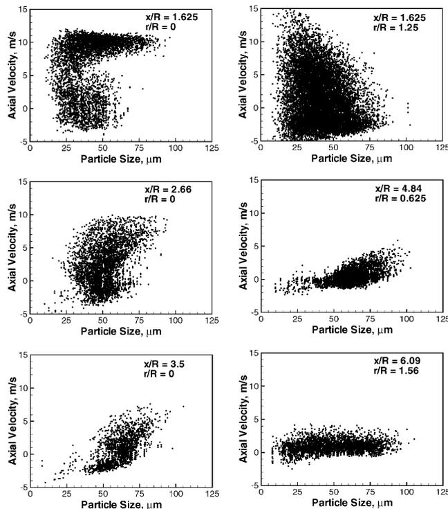
Fig. 12. Particle size-velocity correlations at different locations.
