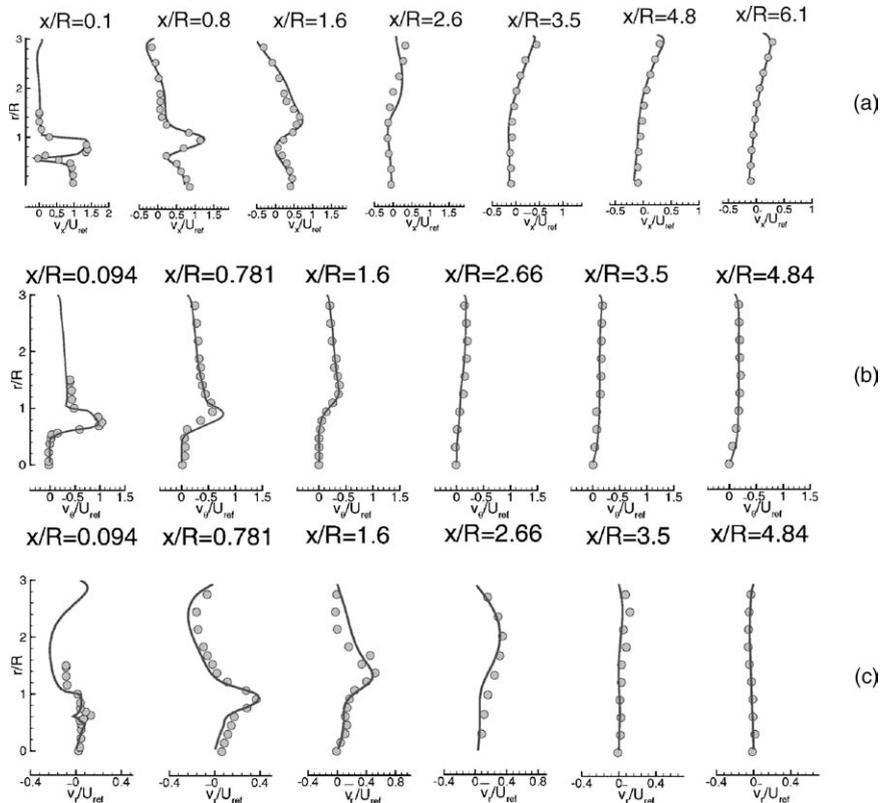
Fig. 6. Comparison of gas-phase properties between LES (—) and experiment ( $\circ$ , Sommerfeld and Qiu, 1991) for swirling flow in a coaxial combustor: (a) mean axial velocity, (b) mean swirl velocity, (c) mean radial velocity, (d) rms of axial velocity, (e) rms of swirl velocity, (f) rms of radial velocity.
