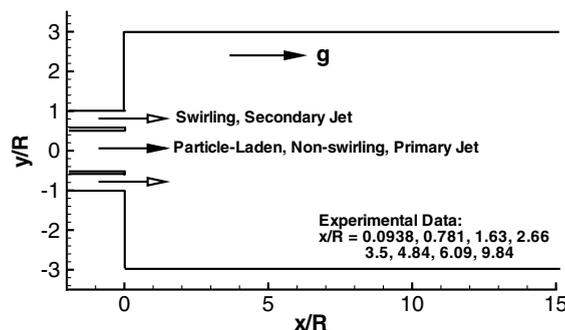
Fig. 1. Schematic of the swirling, coaxial-jet combustor.
