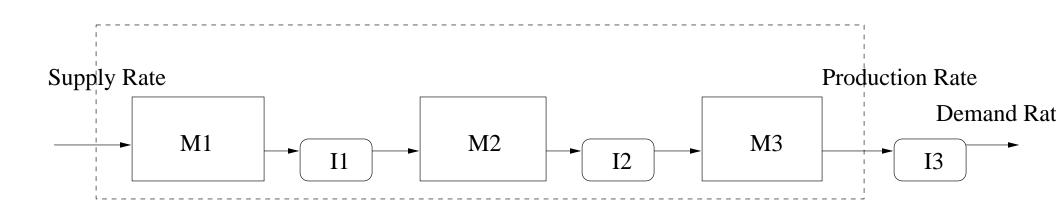
A **transfer line** is a pipeline of manufacturing machines. At each time t, each machine has three possible actions:
