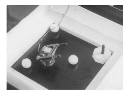
Task: Pick up ball, carry to stick, hit against stick. Sensors: holding-ball, linear vision (stick finder), IR proximity sensors
