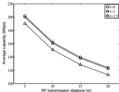
Figure 3: Capacity for different values of  $r$ ;
