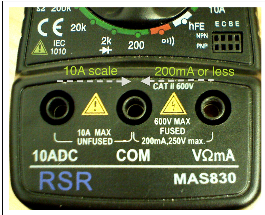
Figure 8: Face of DMM showing imaginary reference current arrows.
