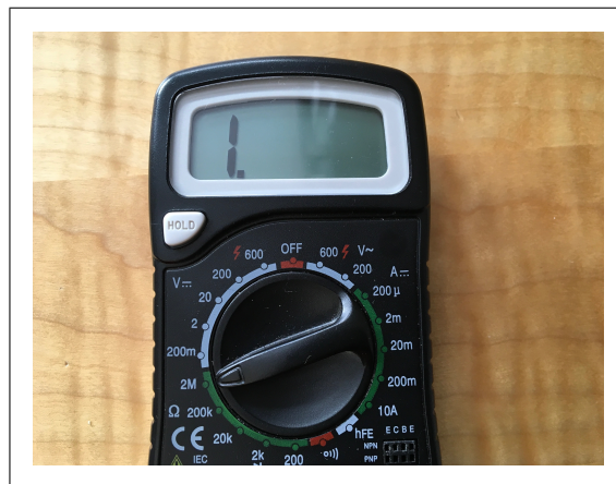
Figure 2: DMM Showing Overrange Resistance Indictation
