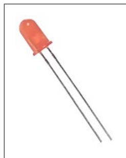
Figure 1: LED - Positive lead (anode) is slightly longer
