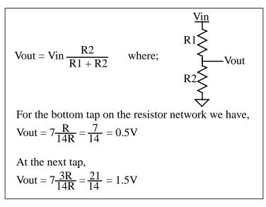
The reference input to each comparator is connected to one of the voltage reference taps. The output of each comparator indicates if the input signal exceeds that reference input.
