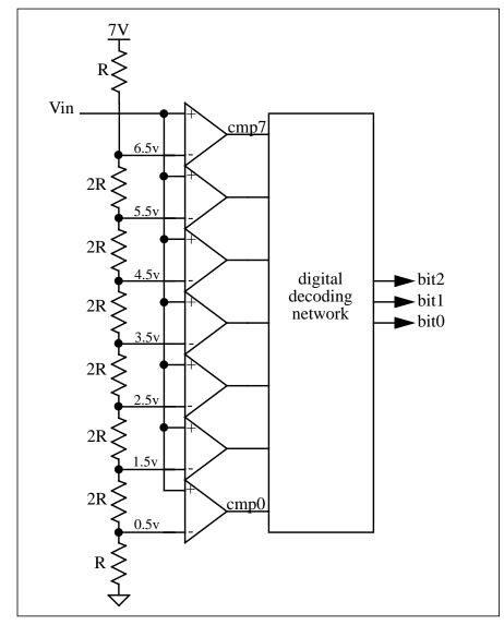
The voltage at the bottom tap follows the voltage divider equation we studied before.
