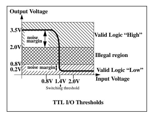
When digital logic has an output voltage of two volts or above its output is considered to be logic "1". An output voltage 0.8 volts or less is considered to be logic "0". Voltages between 0.8 volts and 2.0 volts are considered illegal. The binary logic circuits should never encounter signals within this region except for a quick transition through it when switching states.
