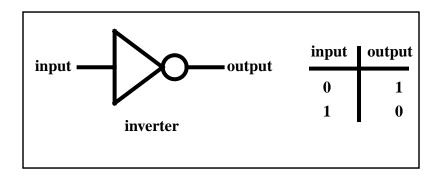
The use of a binary coded signaling system is intentional. First of all, it allows simple implementation with transistor switches that are either "on" or "off". Additionally, the binary system allows us to leverage the work of George Boole and Claude Shannon pertaining to rules for manipulating boolean (logic) variables and thus perform binary arithmetic.
