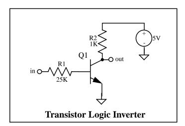
We will adopt the convention that voltages between 2 and 5 volts constitute logic "one" and voltages between 0 and 0.8 volts are logic "zero". Also, assume a transistor beta of 100.
