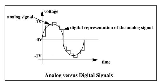
The most interesting system (and the easiest to implement with transistors) is one where a signal my take on only two possible values. These signals are called "binary" signals. We give different names to the binary signal levels; "1" and "0"; "true" and "false"; "on" and "off". These names may represent any particular voltage or current level. Typically, we assign the logic value "1" to the higher output voltage and "0" to the lower output voltage.
