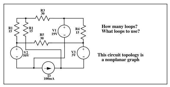
To allow us to easily solve for the voltages and currents, we want the set of independent simultaneous equations with the least number of variables.
