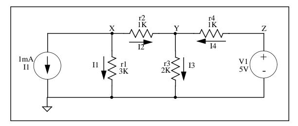
All the nodes have been named and all currents labeled. The common node is the is the ground node which usually appears as a common lead across the bottom of a circuit diagram.
