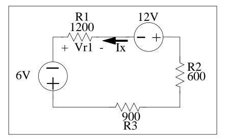
We can see that the 12 volt source is in opposition to the 6v source. Since the 12 volt source is the larger one, it "wins" forcing current to flow out of the positive terminal of the 12 volt source. The effective resultant voltage applied to the circuit is 6v, with the current flows clockwise. Since Ix is shown flowing the opposite way, we know that Ix must be negative.(and it is!)
