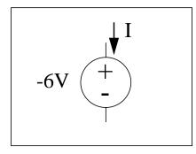
Since the current direction we initially chose is in opposition to the direction that we must show current flowing to the compute power dissipation, so we must change the sign of the magnitude.
