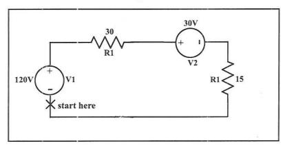
In Spice, circuits are described as "netlists". Netlists are simply a listing of how the elements in the circuit are connected. We describe the connection of the elements by telling which node each terminal of an element is connected to. Therefore, we need to mark the nodes in the circuit with unique node names. These are shown below as the numbers 1,2,3 and the node name "gnd". Note that all Spice netlists must have a ground node in the circuit. The node names are circled for clarity.
