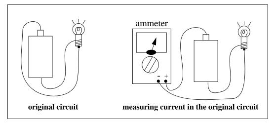
When making measurements, the desire is to make the measurement without disturbing the original circuit. For an ammeter to do this, its internal construction must look much like the portion of the wire it replaced. It is true that the ammeter has a very special calibrated wire inside it that allows a current measurement to be made.
