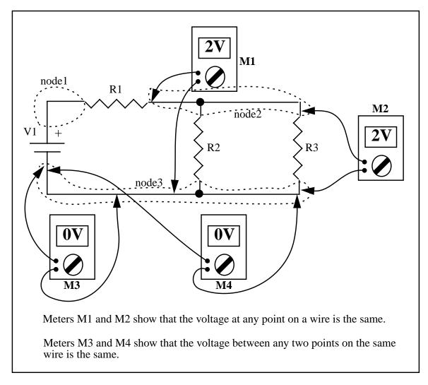
In the drawing the terminology of a *node* is introduced. A node on a schematic circuit is essentially a wire. Thus we can also say that the voltage anywhere on a node is the same. Also it holds that the voltage between any two points on a node is the same.
