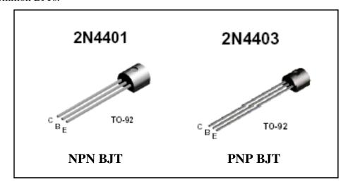
The transistors we will look at are called bipolar junction transistors (BJTs). These transistors are described as *bipolar junction* because they contain two pn-junctions each one like a diode, but arranged back-to-back.
