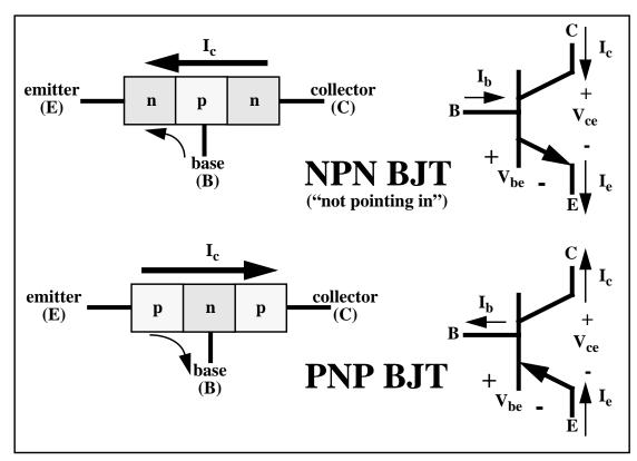
The separate PN junctions can be checked to test a BJT transistor. If the emitter-base, and collector-base junctions each show correct diode behavior, the BJT is not seriously damaged. This is a very simple test, but can form a go-no-go test for the BJT.
