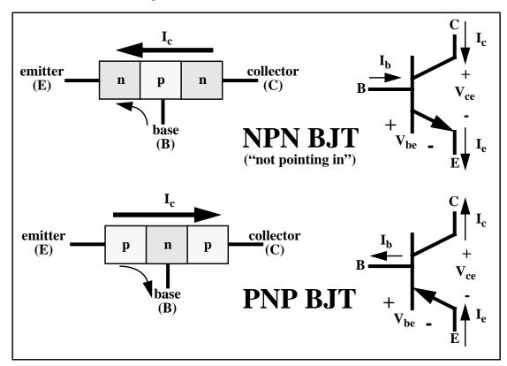
Shown above are the schematic symbols and reference voltage and currents for both NPN and PNP BJTs. Reference voltages and currents are defined identically for both NPN and PNP transistors, even though these symbols represent different types of transistor. You should become familiar with the voltages and currents around the BJT.
