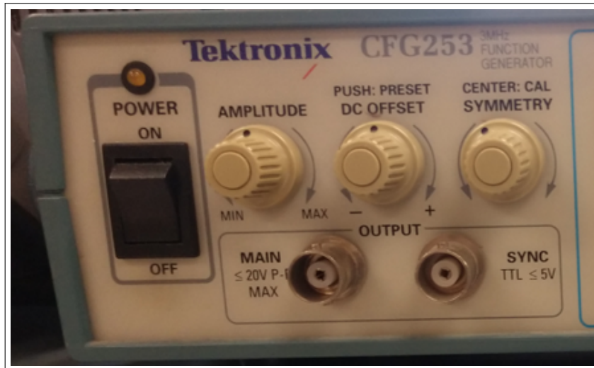
Figure 4: DC Offset Knob on Function Generator
