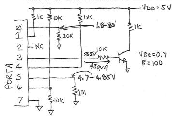
Internal pullups are as stated in the datasheet (20-50K) as well as the logic low and logic high levels (0.2Vdd, 0.6Vdd).
