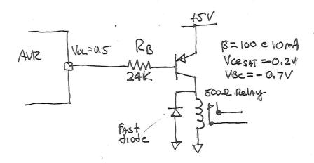
BST must source 10mA to AziAte relay. This will require At teast  $\frac{10mA}{B} = 100\mu A$  of base current. To ensure Saturation assume base current will be 150 $\mu A$ . Thus  $CB = \frac{5-0.7-0.5}{150\times10^{-6}} = 25,333 \Omega$ ; 24K is the runcist value
