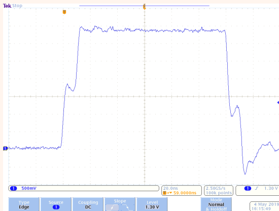
Figure 19: I/O pin driving 50 ohm transmission line
