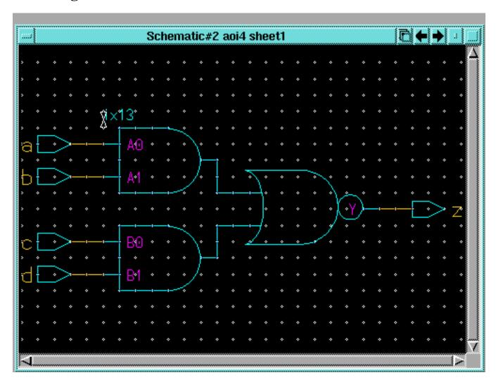
Here we can see the direct correspondence between the gate pins and the entity pins in the statement:
