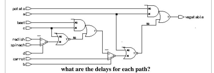
Note how signal with the smallest gate delay through the logic was the first one listed. You can use such behavior to your advantage. Note that use of excessively nested **IF** statements can yield logic with lots of gate delay.
