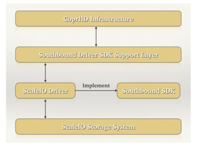
Figure 3.1: Top Level System Architecture
