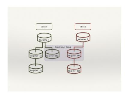
Figure 4.5: Snapshots and Consistency Groups in ScaleIO [7]
