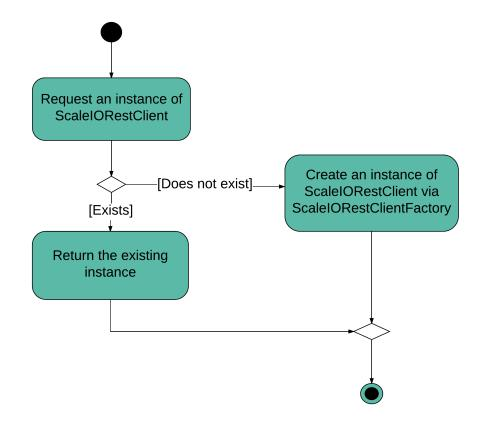
Figure 4.3: Activity Diagram: ScaleIORestClient
