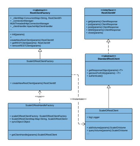
Figure 4.4: ScaleIORestClient Module Class Diagram
