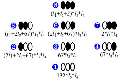
Fig. 2. Cost lattice for the program in Figure 1. We have omitted an addend 2 that is shared by all configurations. The letters  $l_1$ ,  $l_2$ ,  $l_3$ , and  $l_4$ , introduced in Figure 1(a), represent the number of iterations for the respective for loops.
