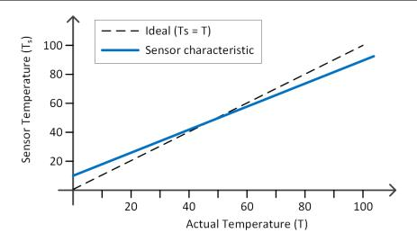
□ Ideally, the sensor temperature,  $T_s$ , would equal the true temperature, T:
