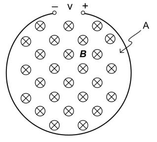
$\bullet \phi$  is the magnetic flux penetrating the coil:
