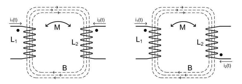
In both cases above, i<sub>1</sub> and i<sub>2</sub> in the directions indicated produce the magnetic flux, B, in same direction
