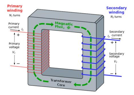
If that flux is time-varying, a voltage is induced across the secondary
