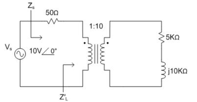
$$V_2 = 79∠18.4^{\circ} V$$
