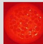
Horizontal slice of Silver Nanoparticles and Polystyrene Beads Resolution 13 µm
