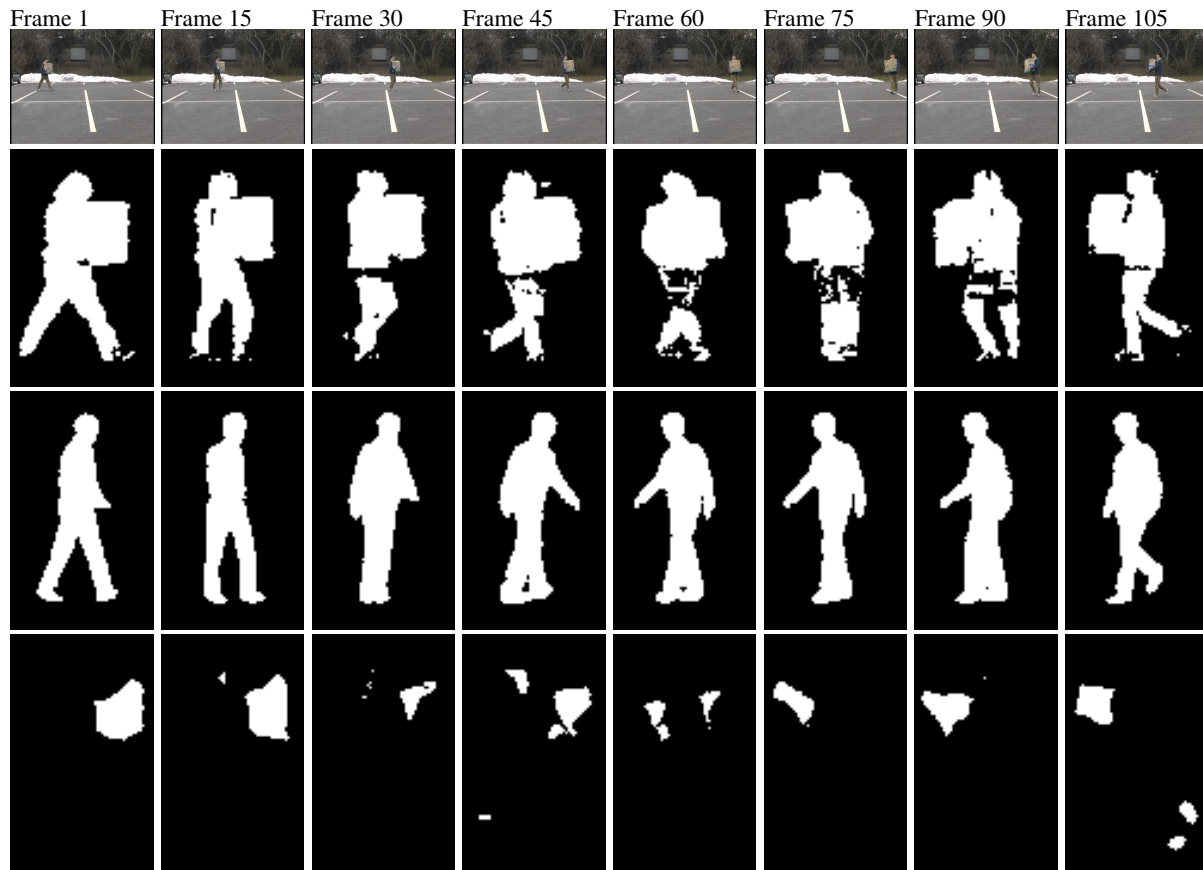
Figure 5. Outlier detection in continuous view variations: First row: Input image. Second row: Extracted silhouette shape. Third row: Best matching shape. Fourth row: Detected carrying object
