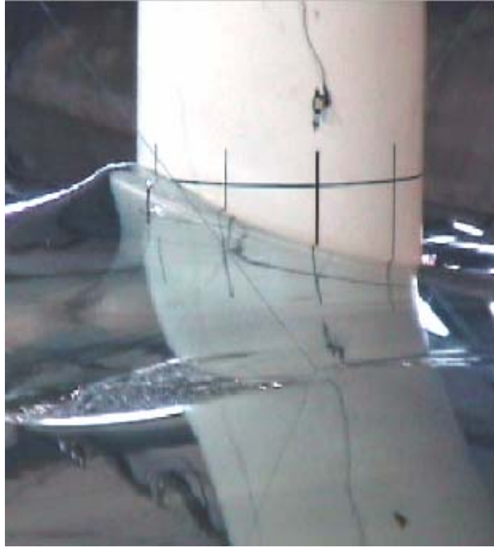
Figure 5 An image of the preliminary experiment for tsunami force on a vertical cylinder. The size of the cylinder is 50 cm in diameter in a water depth of 80 cm.
