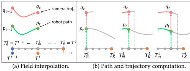
Fig. 4. Field interpolation and path / trajectory computation over time. For a smooth transition from  $T^{t-1}$  to  $T^t$ , we interpolate them with  $K$  sub-steps (small grey dots in (a)), and start to evolve the field from the middle frame  $T_m^t$ . At each sub-step, a smooth robot path (lower grey curve in (b)) is generated by advecting a particle over the current field, along which a camera trajectory (upper grey curve) is computed based on the robot path.
