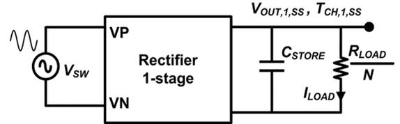
Fig. 5. One-stage equivalent model to estimate  $N$ -stage steady-state output,  $V_{OUT,N,SS}$ , and settling time for a given input swing,  $V_{SW}$ .
