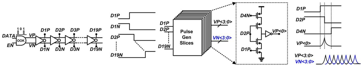
Fig. 13. Generation of UWB pulse with 500-ps pulse width and 8-GHz center frequency using edge combining.
