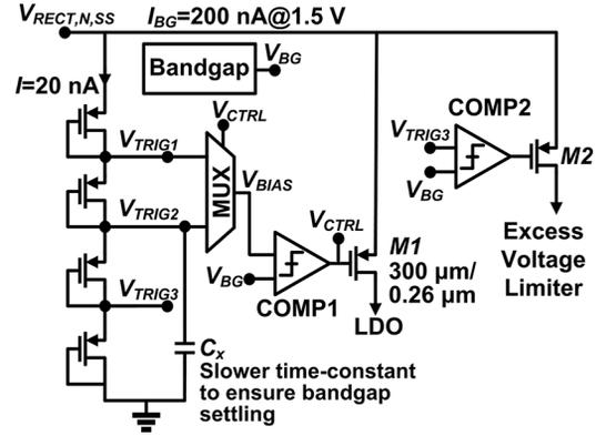
Fig. 12. Schematic of programmable PMU that draws  $< 300$  nA.
