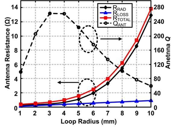
Fig. 7. Loop antenna parameters at 2.4 GHz used in the model in Fig. 3.
