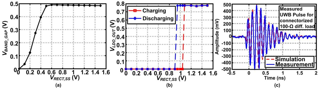
Fig. 21. Measured PMU and 8-GHz UWB TX performance. (a) Low-voltage bandgap operates with  $V_{RECT,SS} > 0.5$  V. (b) Measured LDO output demonstrating constant UWB TX voltage supply as well as appropriate enable/disable during charging and discharging phases. (c) Comparison of simulated and measured 8-GHz UWB pulse when UWB TX is characterized with connectorized 100- $\Omega$  differential load.
