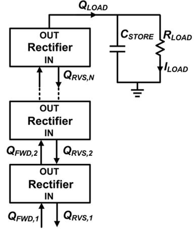
Fig. 4. Charge transfer in the steady state in an  $N$ -stage rectifier.
