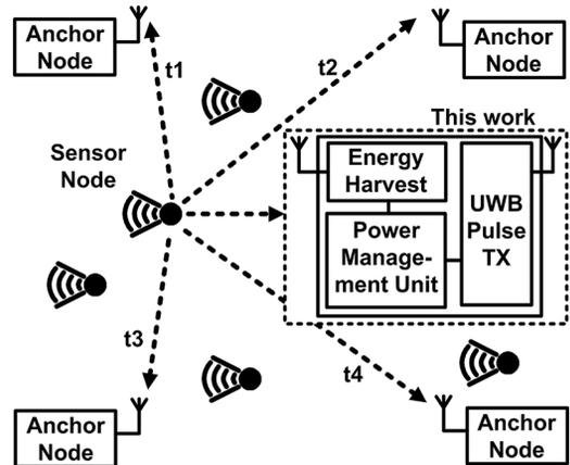
Fig. 1. Relative TDOA-based localization using wirelessly powered UWB TX SoC.
