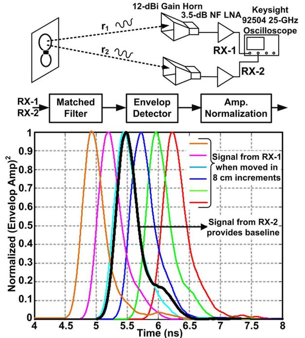
Fig. 24. Relative TOF measurement using the UWB TX. RX-2 provides baseline while the position of RX-1 is varied.
