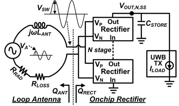
Fig. 3. Circuit and antenna model used to codesign antenna and rectifier for area-constrained sensitivity optimization.
