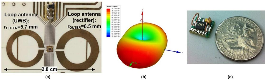
Fig. 15. (a) UWB SoC packaged with dual planar loop-antennas for RF testing. (b) Simulated 2.4-GHz loop antenna gain. (c) Compact 3-D package for low form-factor and weight.
