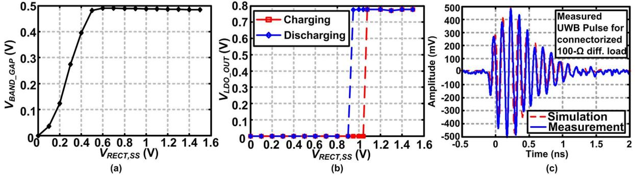
Fig. 21. Measured PMU and 8-GHz UWB TX performance. (a) Low-voltage bandgap operates with  $V_{RECT,SS} > 0.5$  V. (b) Measured LDO output demonstrating constant UWB TX voltage supply as well as appropriate enable/disable during charging and discharging phases. (c) Comparison of simulated and measured 8-GHz UWB pulse when UWB TX is characterized with connectorized 100- $\Omega$  differential load.
