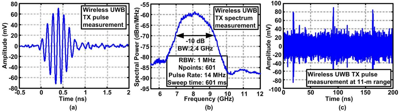
Fig. 22. Wireless measurements of UWB TX in the (a) time domain and (b) frequency domain. Measurements are consistent with 0-dBm UWB TX radiated power. (c) UWB TX pulse achieves  $> 15$ -dB SNR at 11-m range, demonstrating feasibility of operation beyond 10 m.
