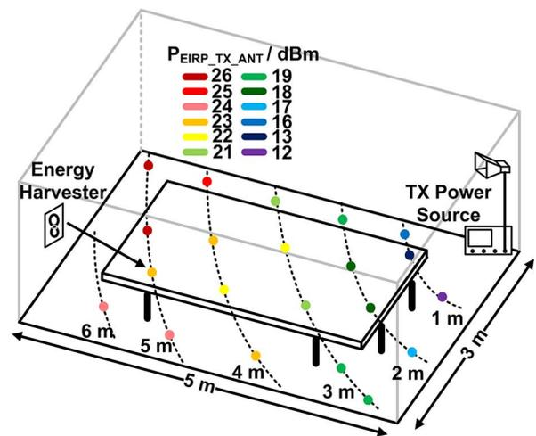
Fig. 20. Diagram of measured 2.4-GHz rectifier performance in a conference room demonstrating feasibility of wireless powering in typical office environments.
