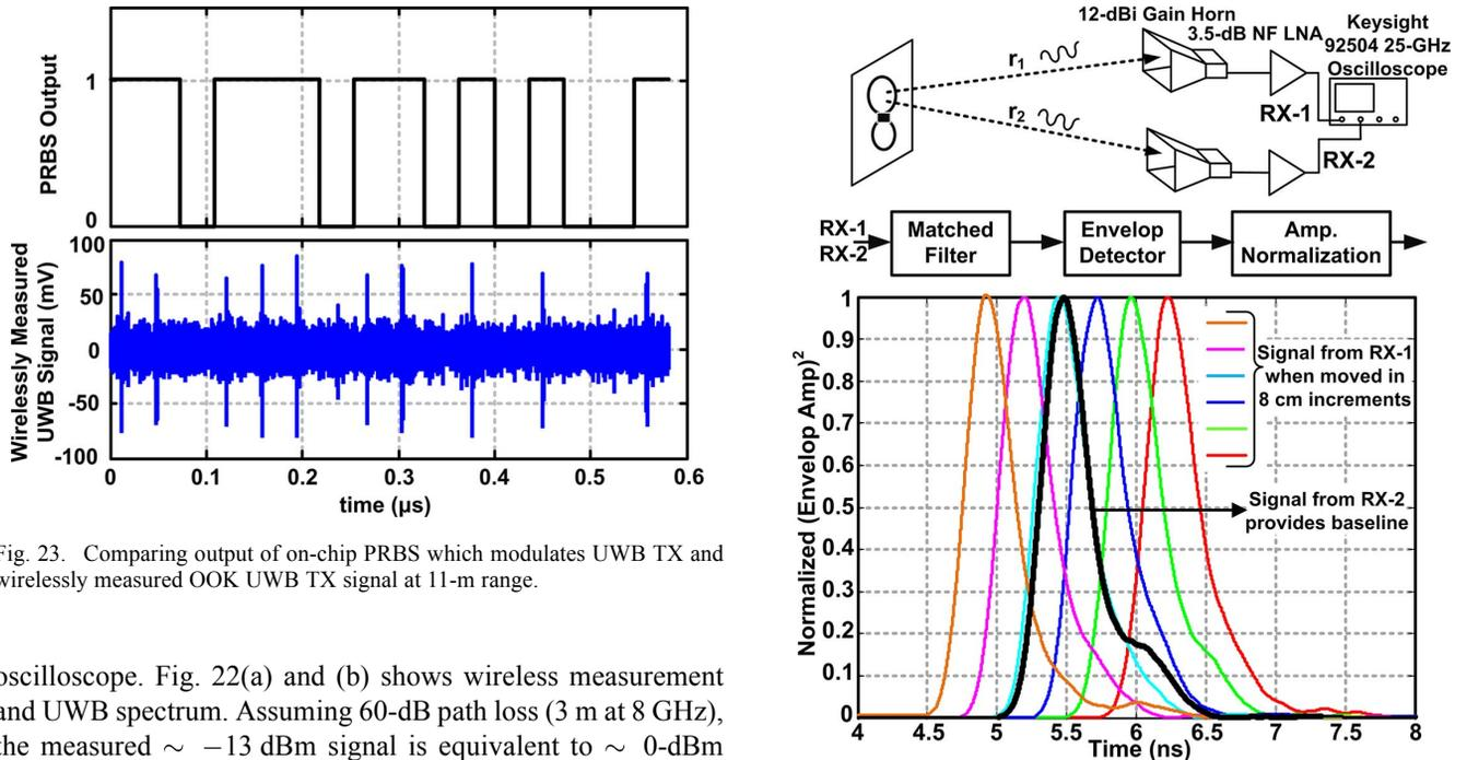
Fig. 23. Comparing output of on-chip PRBS which modulates UWB TX and wirelessly measured OOK UWB TX signal at 11-m range.
