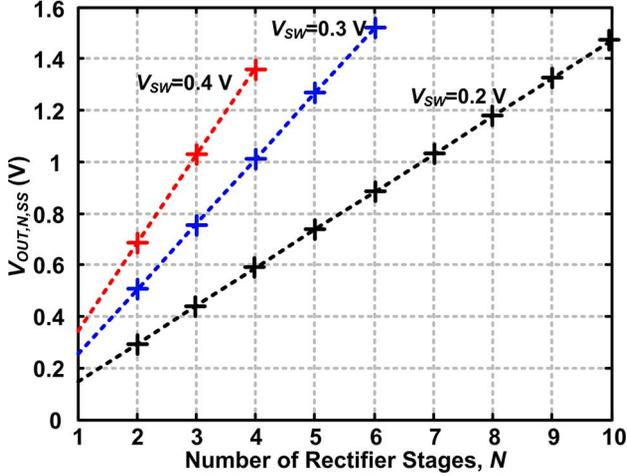
Fig. 6. Comparison between simulated  $V_{OUT,N,SS}$  and estimated  $N \cdot V_{OUT,1,SS}$  from one-stage model shows accuracy of approach.
