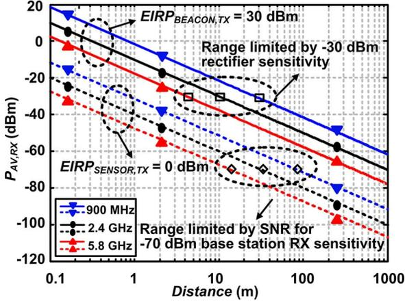
Fig. 2. Wirelessly powered sensor operating range is limited by rectifier sensitivity rather than by the SNR required for the wireless data link between the sensor and base-station.
