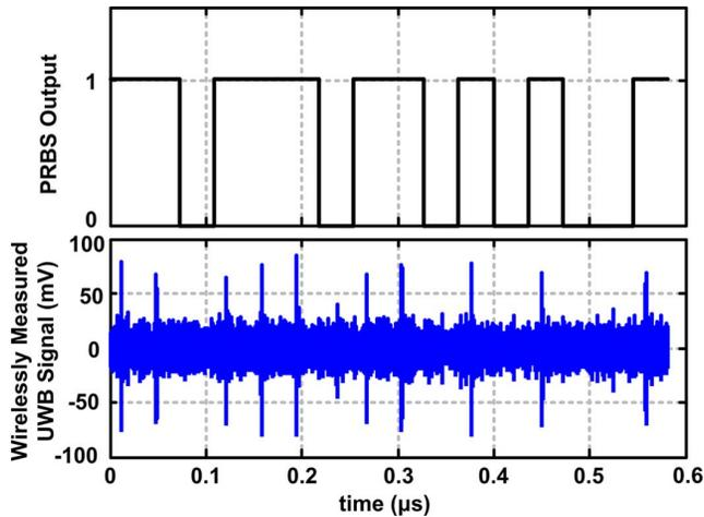
Fig. 23. Comparing output of on-chip PRBS which modulates UWB TX and wirelessly measured OOK UWB TX signal at 11-m range.
