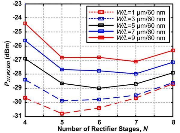
Fig. 10. Required  $P_{AV,RX,ISO}$  to achieve targeted 1-V output voltage across device width and number of rectifier stages.
