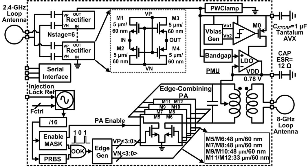
Fig. 11. Wirelessly powered UWB TX SoC with 2.4-GHz rectifier, low-current PMU, and 0.8-V 8-GHz UWB TX.
