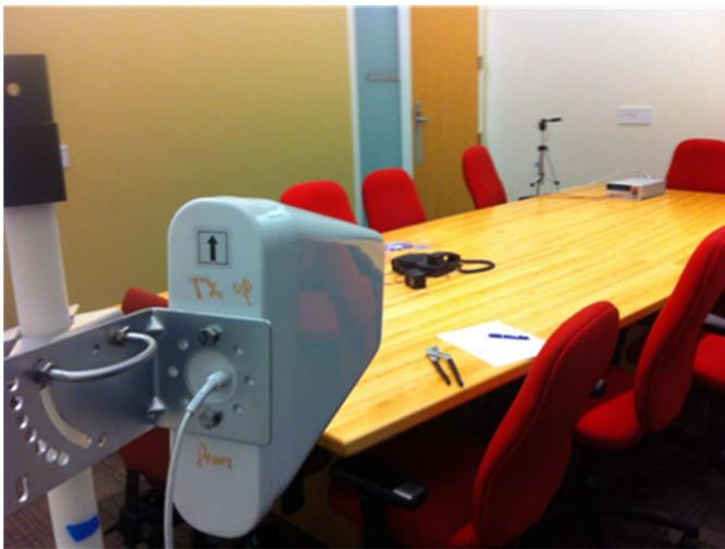
Fig. 19. Photograph of a 2.4-GHz rectifier-antenna characterization in a typical office conference room.
