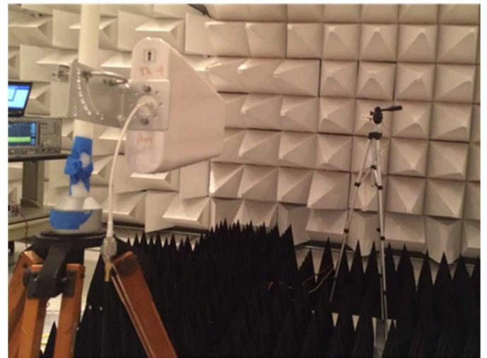
Fig. 17. Photograph of a 2.4-GHz rectifier–antenna measurement in an anechoic chamber.
