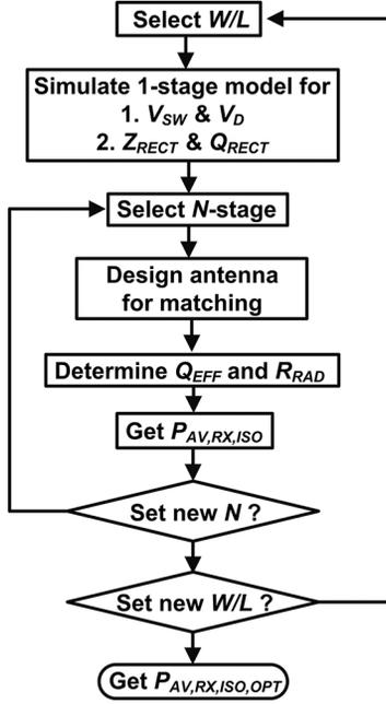
Fig. 8. Systematic rectifier–antenna codesign for optimizing rectifier sensitivity.
