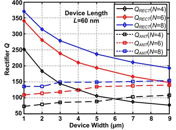
Fig. 9. Rectifier and antenna quality factors following codesign approach in Fig. 8, satisfying 1-V output voltage target.
