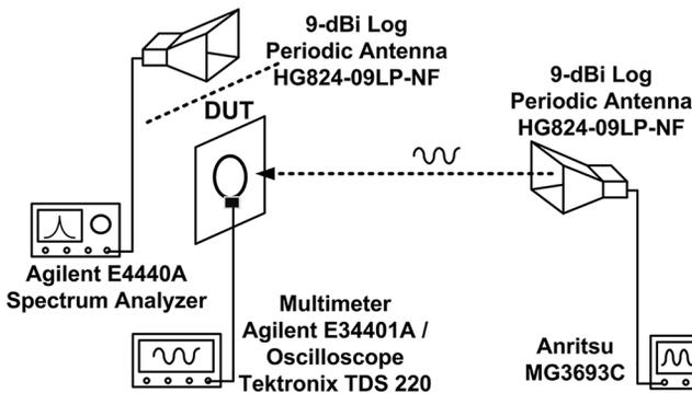
Fig. 16. Measurement setup for characterizing rectifier performance—setup is initially calibrated to determine available power for the rectifier.
