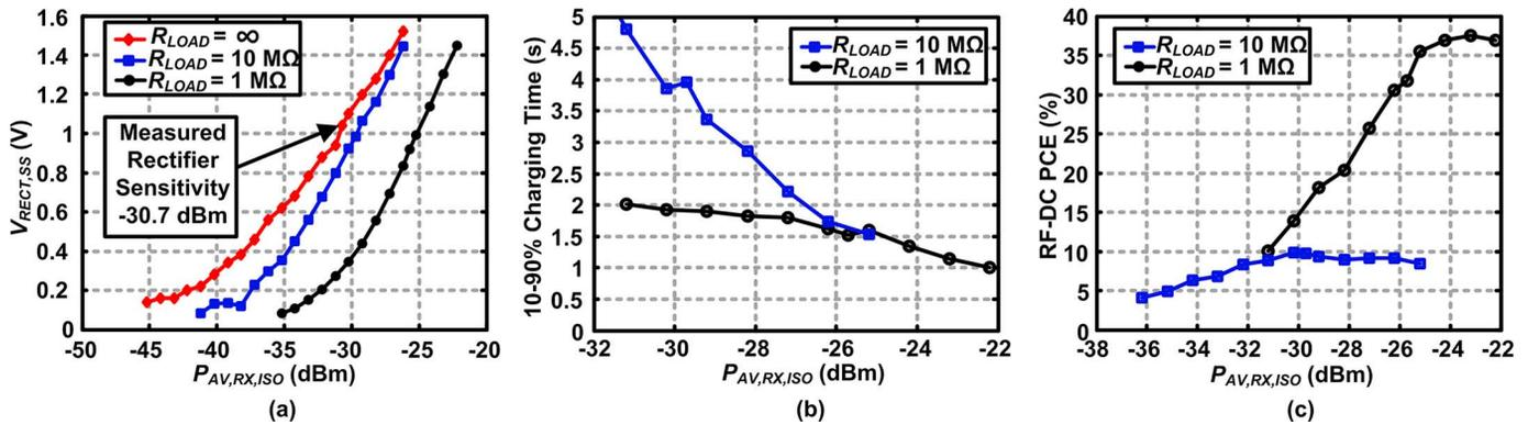
Fig. 18. Measured 2.4-GHz rectifier performance. (a) Rectifier sensitivity across target output voltage and  $R_{LOAD}$ . (b) Rectifier charging time for 1- $\mu\text{F}$  storage capacitor. (c) Rectifier PCE across input power for  $R_{LOAD} = 1\text{ M}\Omega$  and  $10\text{ M}\Omega$ .
