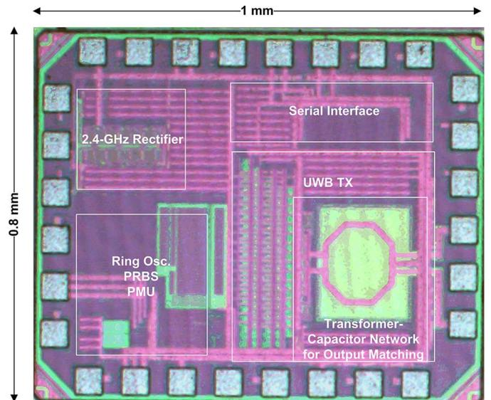
Fig. 14. Die photograph of wirelessly powered 8-GHz UWB TX implemented in 65-nm CMOS.
