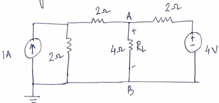
To calculate the Thevenin voltage,  $R_L$  is removed and the voltage  $V_{AB}$  is calculated.
