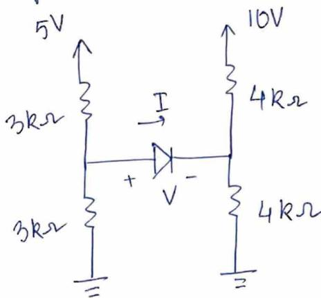
Applying Thevenin's theorem to the left hand side of the circuit,
