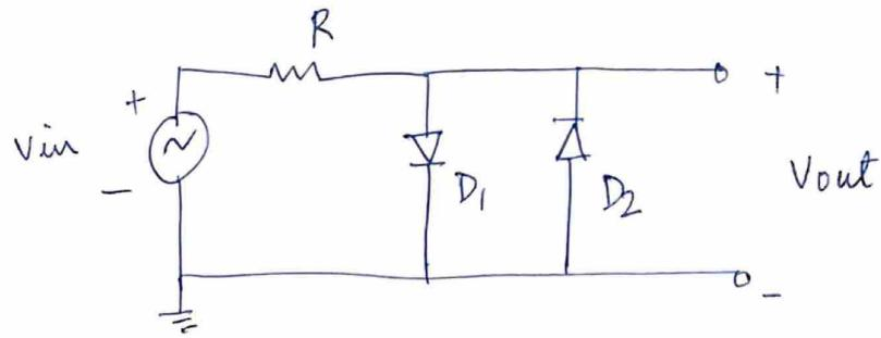
Region 1:  $V_{in} > 0.7V \Rightarrow D_1$  is forward biased.  $\Rightarrow V_{out} = 0.7V$
