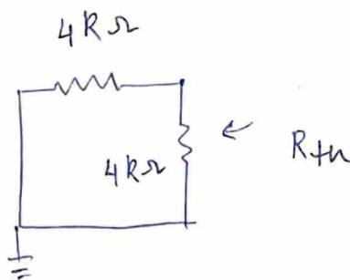
$$R_{th} = (4\text{ k}\Omega \parallel 4\text{ k}\Omega) \\ = 2\text{ k}\Omega$$
