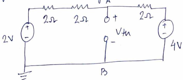
$$\begin{aligned} V_{th} &= 4V - \frac{(4-2)V}{6\Omega} \times 2\Omega \\ &= \frac{10V}{3} \end{aligned}$$
