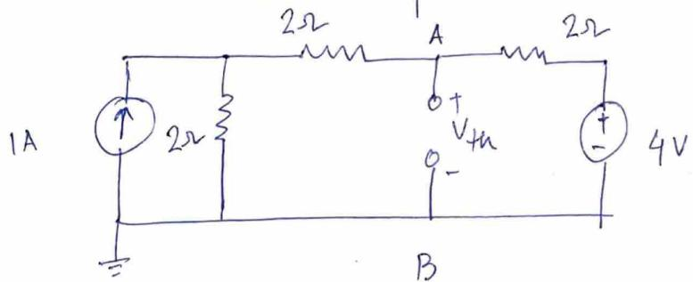
The Thevenin voltage can be calculated using different methods (Source transformation, KCL, KVL etc)
