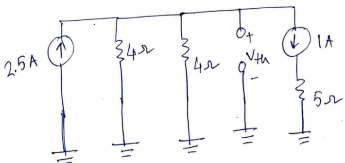
$$V_{th} = (2.5A - 1A)(4\Omega \parallel 4\Omega) = (1.5A)(2\Omega) = 3V$$
