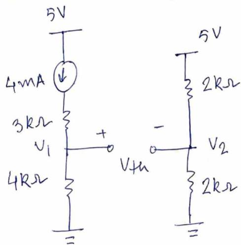
$$V_{th} = V_1 - V_2$$
