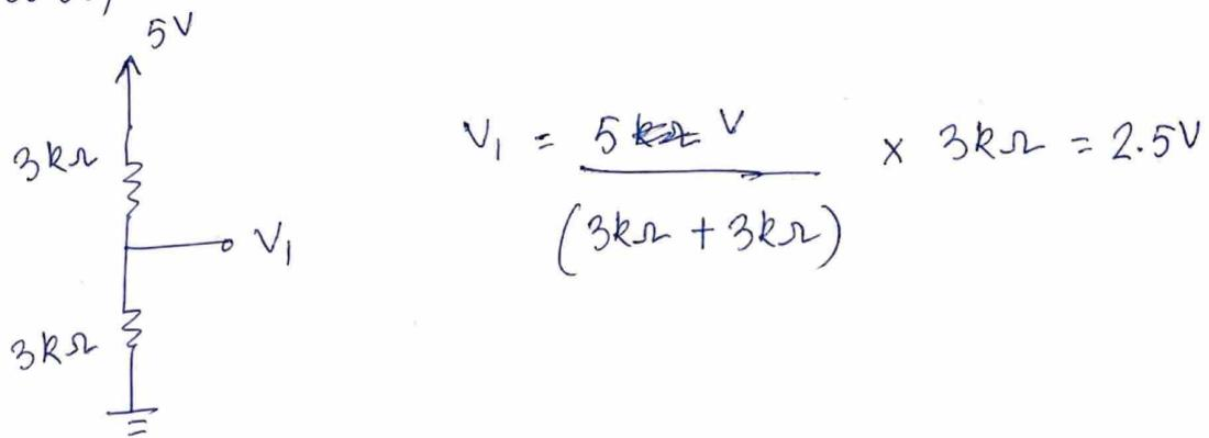
For calculating  $R_{Th}$  for the left hand side of the circuit,
