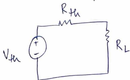
$$V_{th} = \frac{10}{3} V, R_{th} = \frac{4}{3} \Omega, R_L = 4\Omega$$
