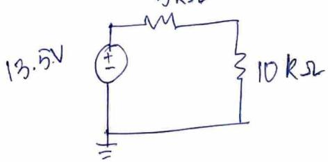
$$V_0 = \frac{13.5\text{V}}{(5\text{k}\Omega + 10\text{k}\Omega)} \times 10\text{k}\Omega = 9\text{V}$$
