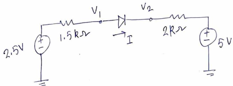
Since  $V_1 < V_2$ , the diode is reverse biased.  $I = 0$
