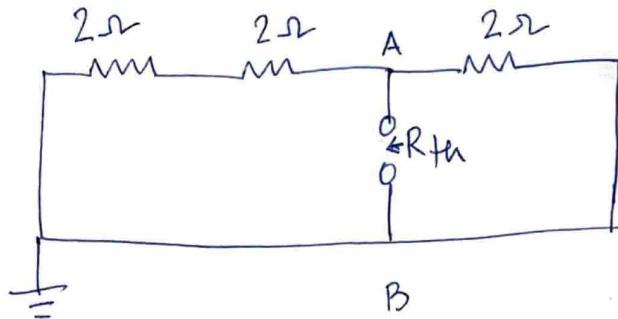
$$R_{th} = R_{AB} = 4\Omega \parallel 2\Omega = \frac{4}{3}\Omega$$
