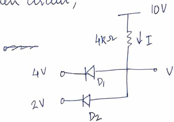
Since the value of the voltage  $V$  is unknown, we cannot estimate the operating condition of  $D_1$  and  $D_2$  intuitively.
