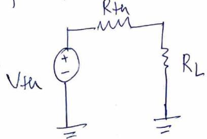
$$V_{th} = 3V, R_{th} = 2\Omega, R_L = 2\Omega$$
