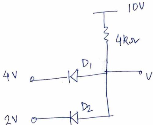
For real diodes, voltage drop across the diode in forward biased = 0.7V
