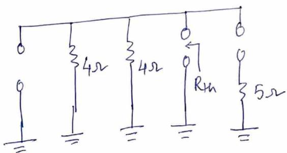
$$R_{th} = (4\Omega \parallel 4\Omega) = 2\Omega$$
