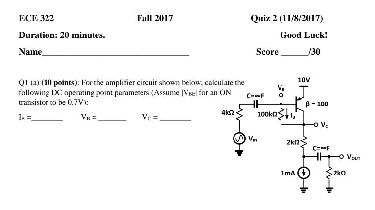
(b) (10points): Calculate the following small signal parameters (assume Vth = 25mV):
