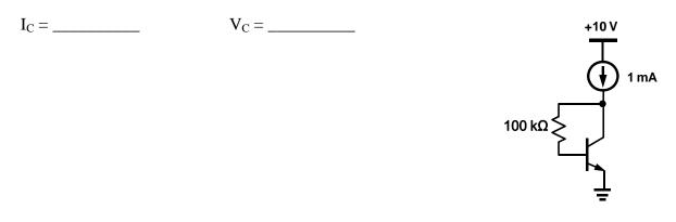
c) For the circuit shown <u>determine</u> the region of operation (cutoff, active, or saturation) for the transistor with  $\beta = 49$ . (15 points).
