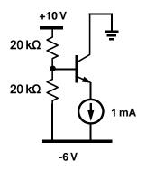
4. For the circuit shown, the emitter voltage is 4 V. <u>Calculate</u> the collector voltage and collector, base, and emitter currents for the transistor. Use this information to <u>calculate</u>  $\alpha$  and  $\beta$ . **Do not assume large**  $\beta$ .  $|V_{BE}| = 0.7V$  for an ON transistor. (25 points).
