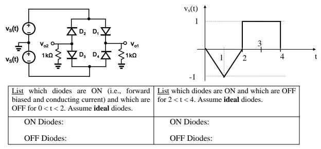
2. Consider the diode circuit shown below with a signal voltage waveform  $v_s(t)$  as shown. Draw the specified voltage waveforms in the table below. (25 points).
