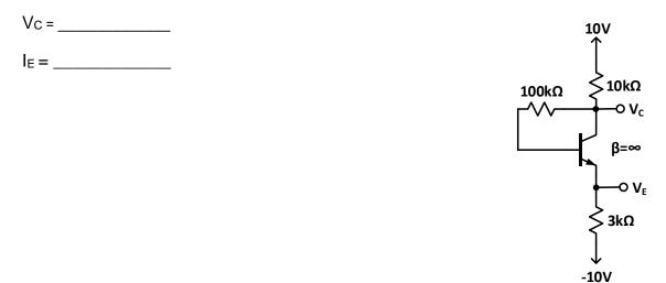
(c) For the circuit shown below, assume  $|V_{BE}| = 0.7V$ , determine the region of operation for the transistor (cutoff, active, or saturation) and calculate Vc
