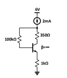
**Problem 4: (30 points)** For the circuit shown below  $|V_{BE}| = 0.7V$ , <u>calculate</u> the following quantities:
