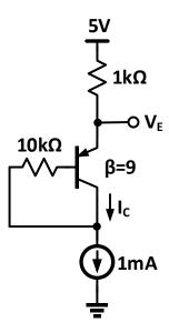
(c) For the circuit shown below, assume  $|V_{BE}| = 0.7V$ , <u>determine</u> the region of operation for the transistor (cutoff, active, or saturation)
