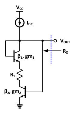
**Bonus (10 points)** For circuit shown below, <u>draw the small signal model</u> and <u>derive the small signal resistance</u>  $R_{\rm IN}$ .
