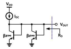
**Problem 2: (20 points)** For circuit shown below, <u>draw the small signal model</u> and <u>derive the small signal resistance</u>  $R_0$ .
