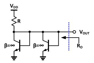
(b) (10 points): For circuit shown below, <u>draw the small signal model</u> and <u>derive the small signal resistance</u>  $R_O$ . The current gain  $\beta$  is finite. Both the BJTs are similar. Assume transconductance of both the BJTs = gm.
