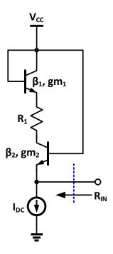
**Problem 3: (20 points)** For the amplifier circuit shown below, calculate the amplifier gain  $V_{OUT}/V_{IN}$  through small signal analysis (show the complete analysis). Assume  $|V_{BE}|$ =0.7V
