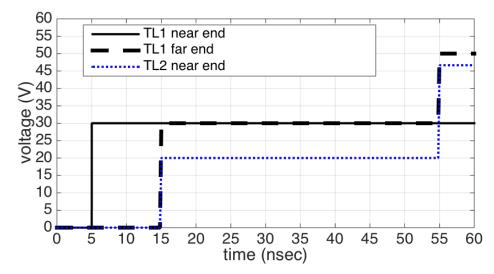
(a) Determine the delay times TD1 and TD2 of the two PCB traces TL1 and TL2, respectively.
