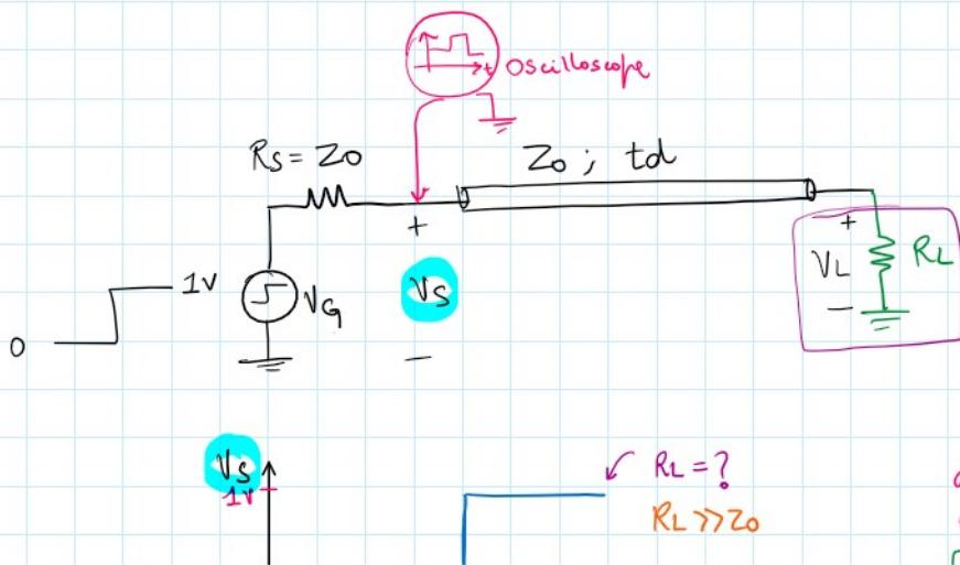
How to know the load by observing the voltage V\_s.
